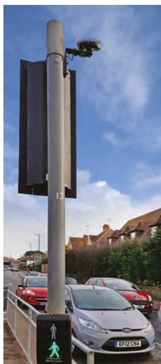
Above: The 645 detects targets in larger zones with 3D HD stereo optics
