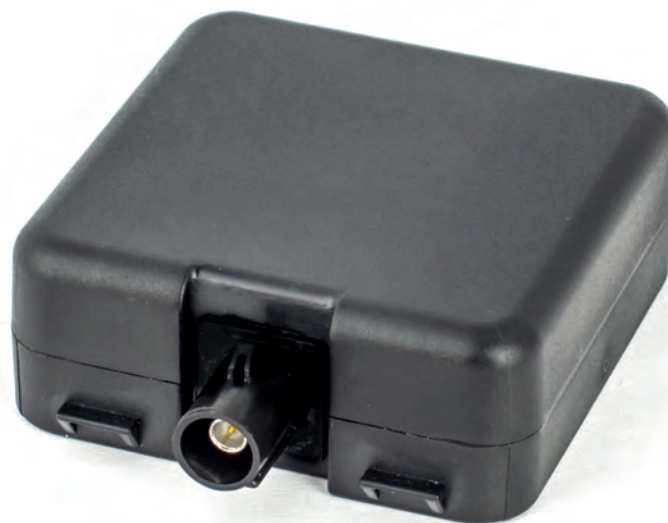
Left: Norbit ITS's detached antenna for smart tachographs Below: The DSRC CAN acts as a DSRC server in the truck
