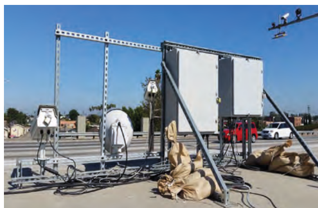
Far left and left: The pilot installation of an automatic vehicle occupancy detection system that LA Metro undertook in partnership with Conduent
