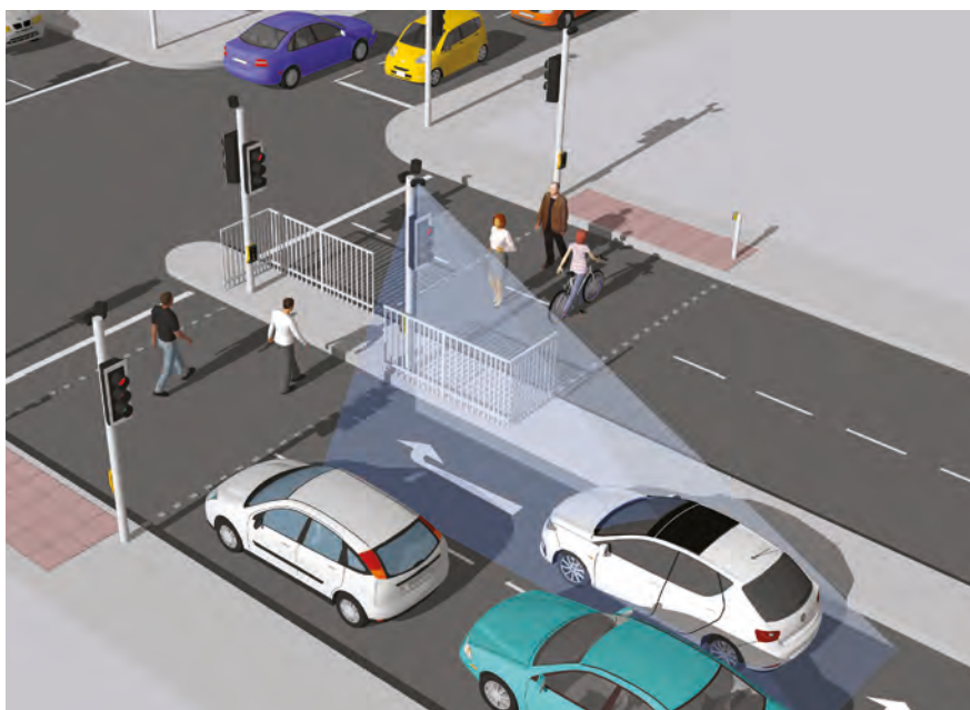
Left: The IP-capable AGD 645 detects right-hand turning vehicles at the stop line
