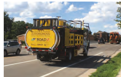
Left: The autonomous attenuator truck relies partly on GPS data from the vehicle ahead of it for navigation
