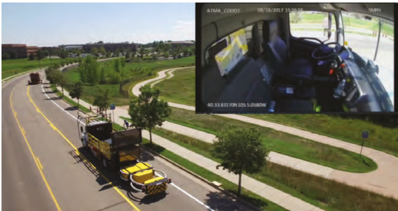
Left: The autonomous attenuator truck relies partly on GPS data from the vehicle ahead of it for navigation
