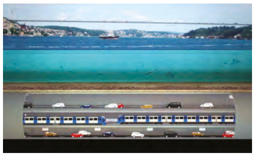
Below: When completed, the Grand Istanbul Tunnel will be the world's first three-story tunnel
