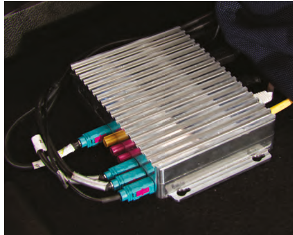
Left: One of the vehicle OBUs used in the Connected Vehicle Pilot in Tampa, Florida. Some volunteers have complained they are unsightly
