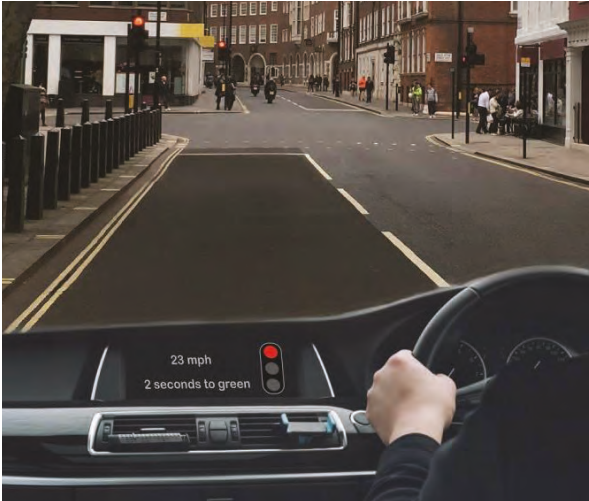
Above: Traffic light phase and timing information can be sent directly to vehicles to aid smoother driving
