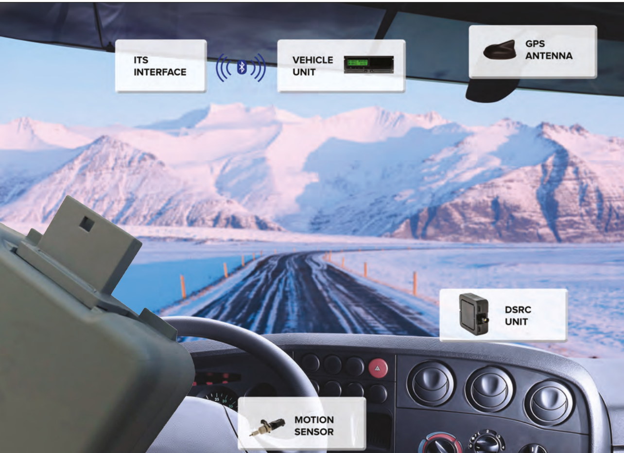
Left: The elements inside of trucks that enable smart tachograph use Inset: The DSRC CAN can be used independently from the smart tachograph
