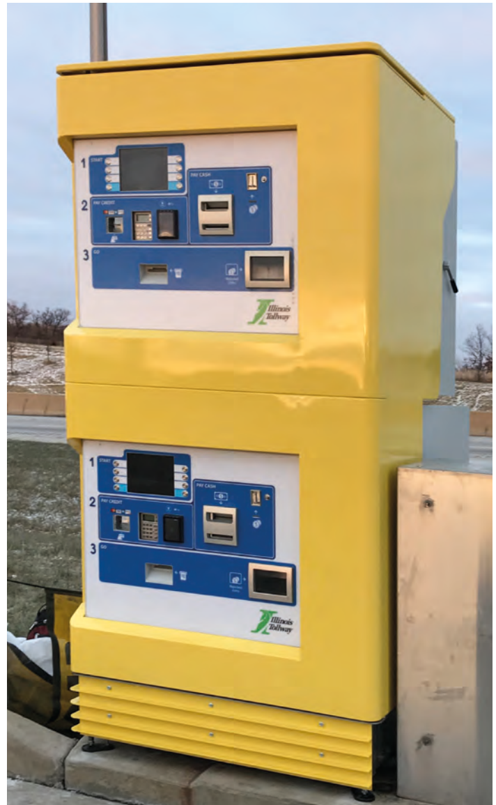
Left: Automatic toll payment machines (ATPM) – such as these in Virginia's Pocahontas Parkway – allow road users to pay for tolls using any means of payment
