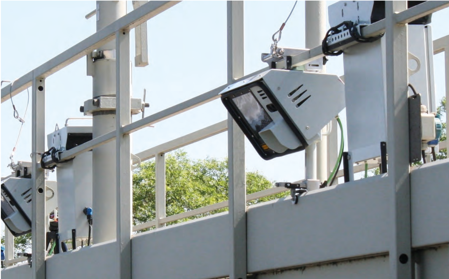
Above: The Portable Label Check verifies the validity of vignette stickers on cars
