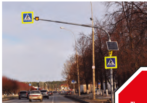
Above: Solar-powered lights are proving useful on rural roads not connected to the power grid Left: Solar signaled crossings in Russia are equipped with pedestrian motion sensors
