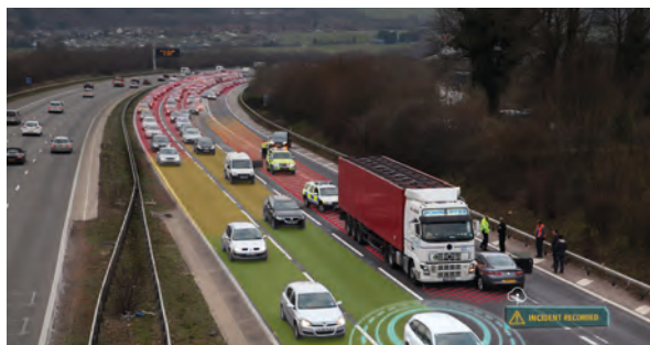
Left: When an incident occurs out of the view of a traffic camera, probe data provides the best way to report it to traffic managers
