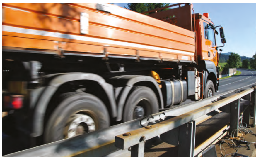
Left: The iBWIM device can collect vehicle load data from a particular bridge over timespans of days or years
