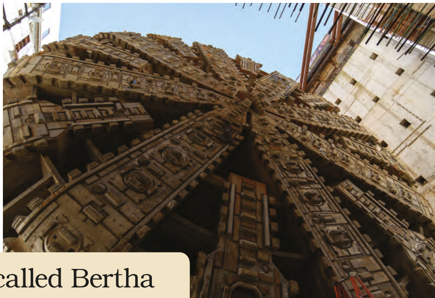
Above: Bertha, the largest tunneling machine in the world at the time, bored the ground to create the foundation for the new SR 99 tunnel
