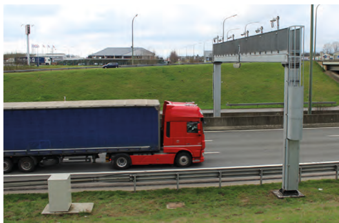
The Global-WIM system measures vehicle characteristics including the license plate number, gross weight and axle load, speed and length
