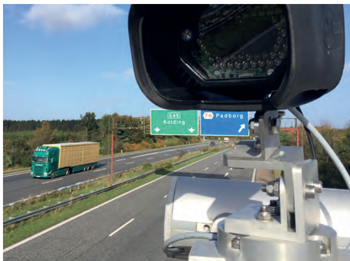
Above: An ALPR and overview camera with integral infrared LED
