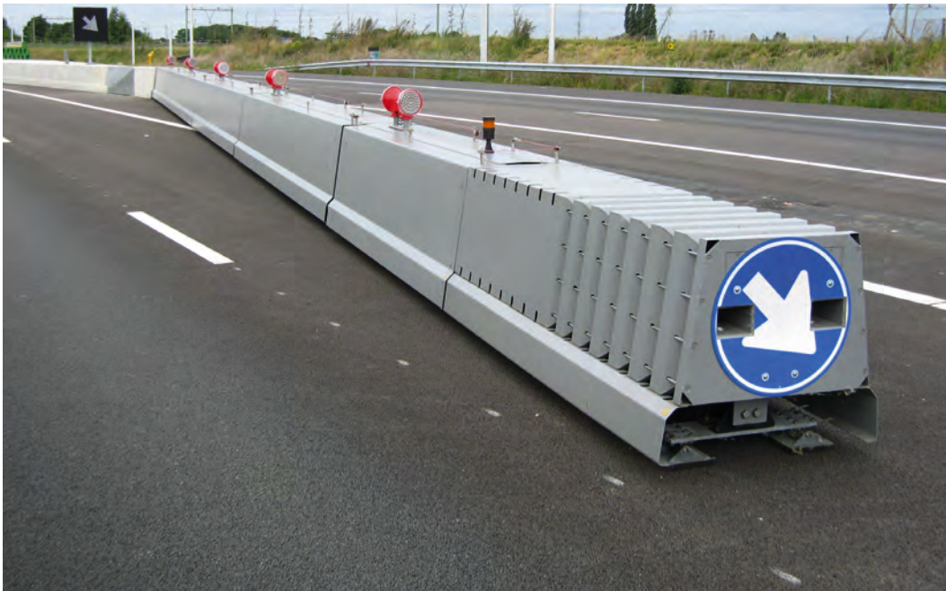
Far left and left: The old barrier system, which could be moved manually with a pickup truck, required staff to be on-site in hazardous conditions
