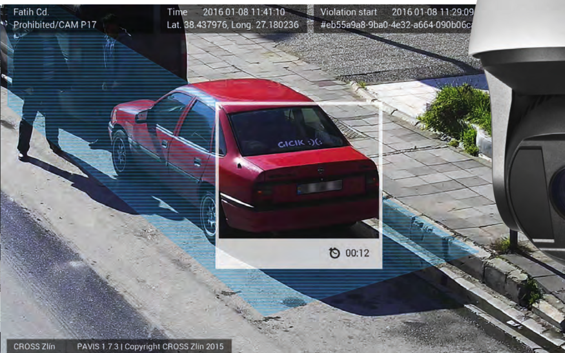
Above: PAVIS uses pan-tilt-zoom (PTZ) cameras to monitor parking and non-parking areas
