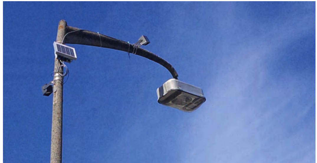
Above: The BS2-TS is an easy to install solar-powered traffic data collection unit
