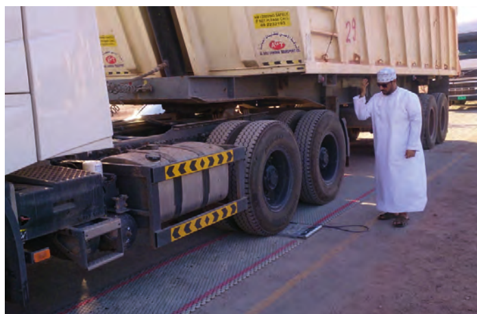
Above: A truck being weighed in Oman with a portable weighing system
