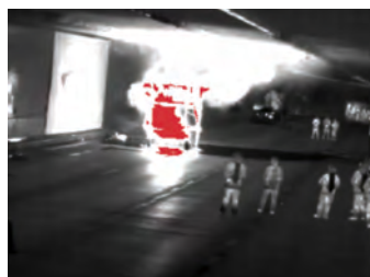
Above: An early-stage tunnel fire is detected by a Flir thermal imaging camera
