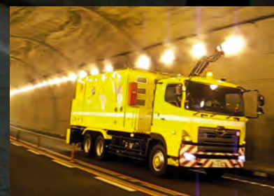
Above: The cavitation jet, high-speed cleaner system, developed by the Central Nippon Expressway maintenance team in Japan
