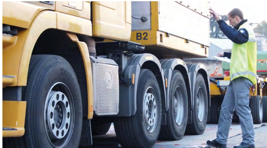
Static weighing of a special transport after detecting overloading with SiWIM
