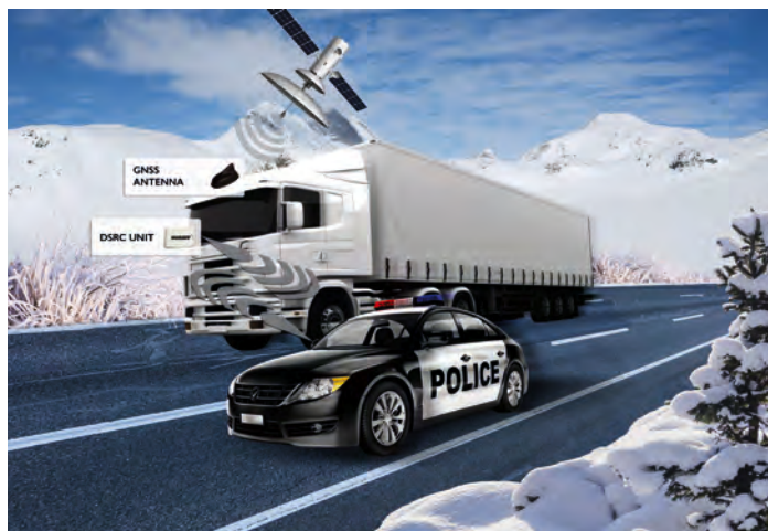
Left: The smart tachograph also communicates with GNSS to record a vehicle's location and is connectable via Bluetooth
