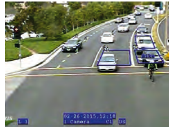
SmartCycle detects bicycles at intersections and can help adjust traffic signal green time accordingly
