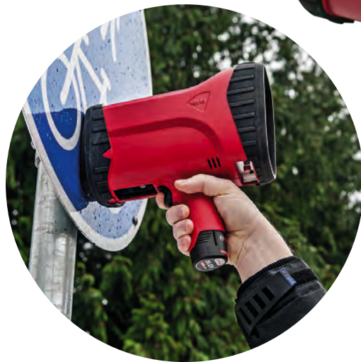
(Above and left) The new RetroSign GRX can capture seven observation angles in a single measurement
