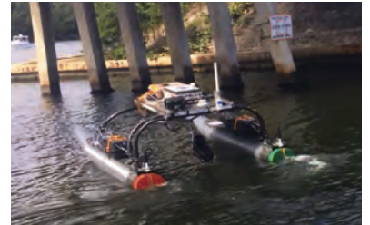
(Below) An unmanned surface vehicle can 'see' bridge footings through silt, sediment, debris and algae
