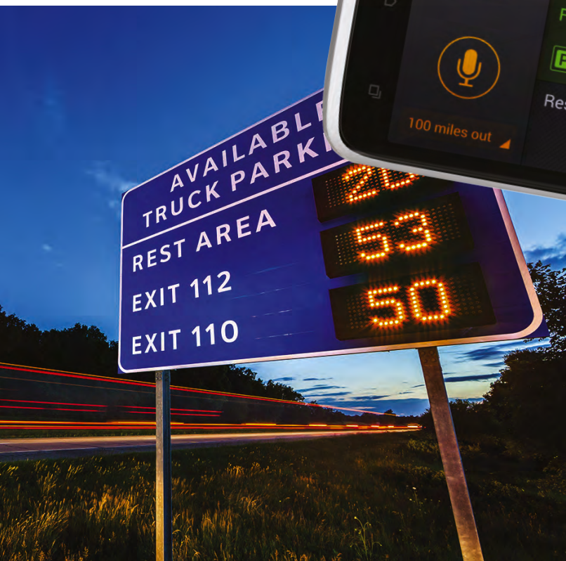
(Above and left) TSPS provides parking availability data on roadside VMS and via an easy-to-use smartphone app
