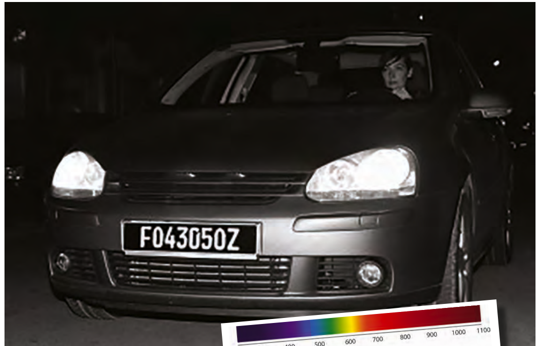
(Above) Driver detection using NIR (Right) UV to NIR Spectrum
