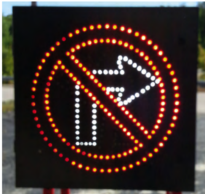
A single sign can be used for multiple messages, such as a 'no right turn' sign (left) or a pedestrian crossing signal (below) – achieving the functionality of traditional dynamic message signs at a much more affordable cost
