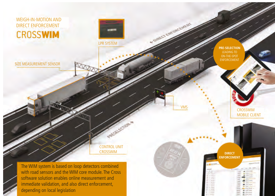
(Left) CrossWIM can be used for both preselection and direct enforcement (Below left) A CrossWIM system in situ in Korea
