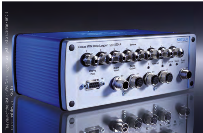
(Above) Kistler's WIM data logger (Right) The Lineas quartz WIM sensor
