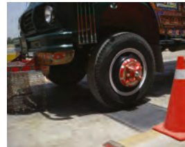
(Above and right) In Pakistan, high-speed WIM is not an option due to the associated costs, but some low-speed applications are in place
