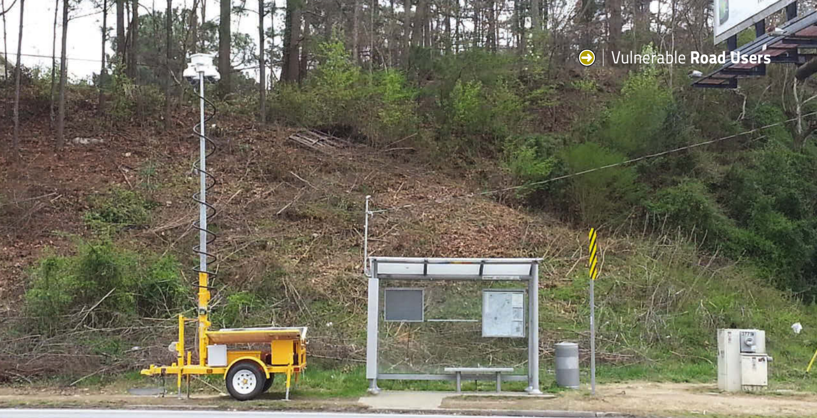
Georgia Tech's mobile machine-vision unit has high-definition cameras that are solar powered
