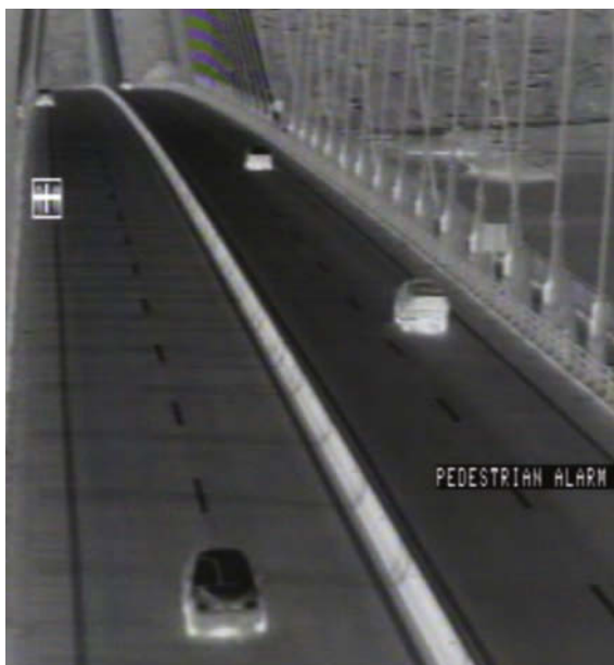
(Left) The latest thermal imaging can distinguish vehicles from pedestrians – key at border crossings
