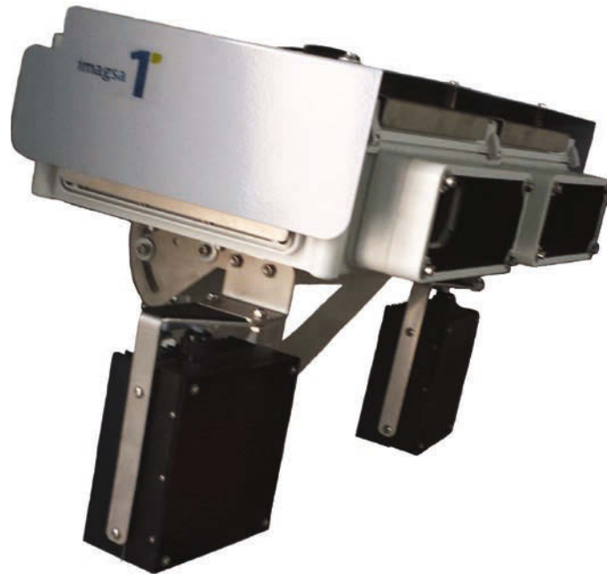
(Left) The stereoscopic vision in Imagsa's Chronos'Spot can analyze 1080 megapixels per second
