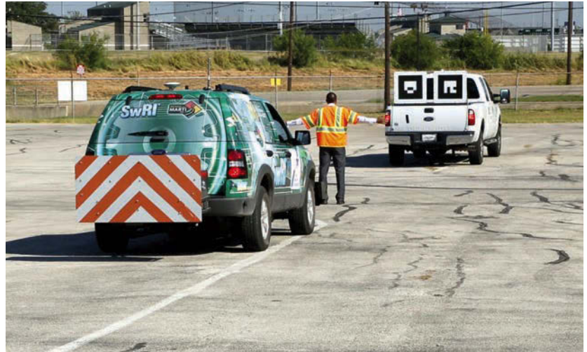
(Above) The prototype attenuator truck, developed by San Antonio's Southwest Research Institute, is completely driverless
