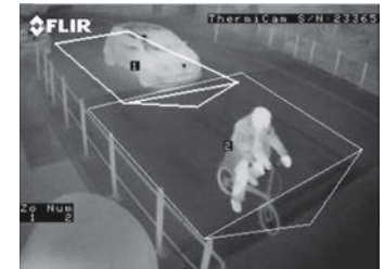
(Top and above) FLIR's ThermiCam detects heat emitted from all types of road users
