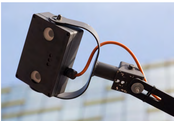
(Below) Transport for London’s SCOOT system is now being expanded to include machine vision that detects numbers of pedestrians waiting at crossings
