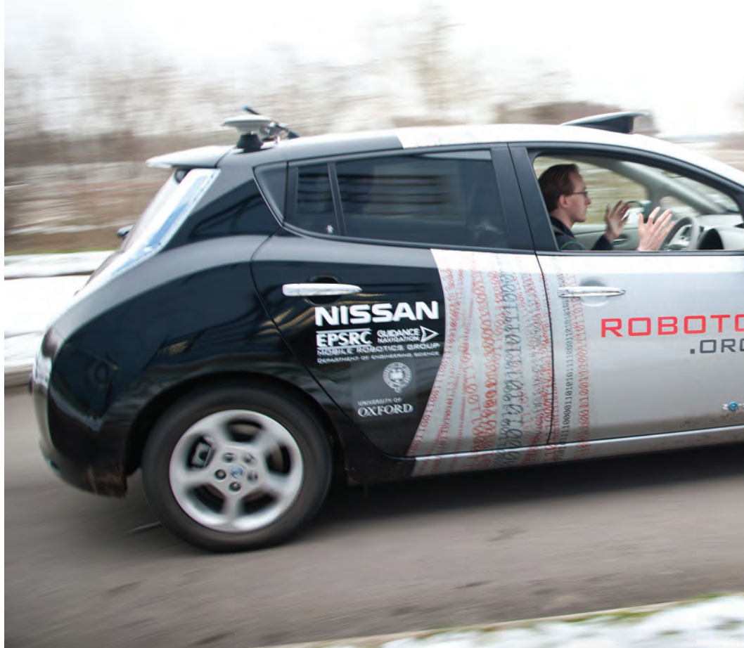
(Above) Oxford University’s RobotCar project navigates using on-board ‘plastic’ mapping techniques
