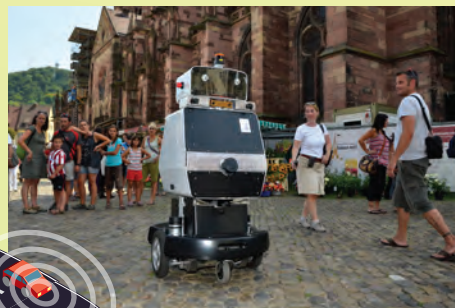
(Above) Obelix, a robot created by the University of Freiburg, Germany, autonomously maps its way through the city's streets
