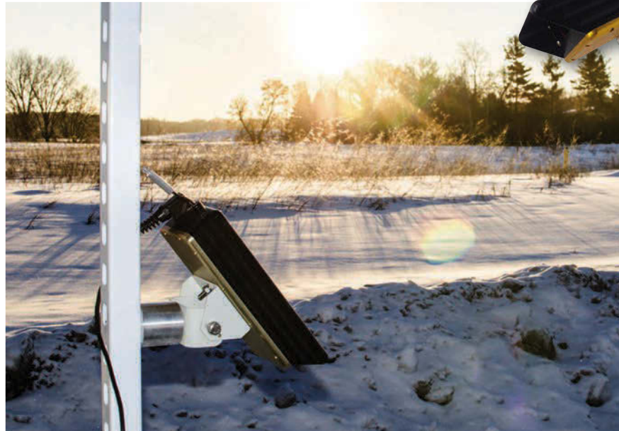
(Above) The Model 5435 Mobile IceSight remote surface condition sensor (Left) Mobile IceSight testing in Minnesota
