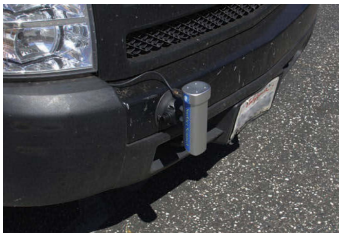
(Left) The Model 5436 Mobile Surface Sentinel surface temperature sensor
