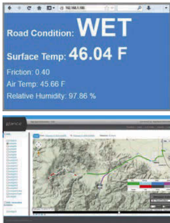
(Top) The Mobile IceSight dash display (Above) Glance visualization software to display mobile weather data
