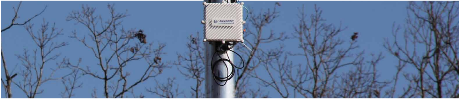
(Above) DSRC-enabled roadside units connect vehicles to infrastructure
