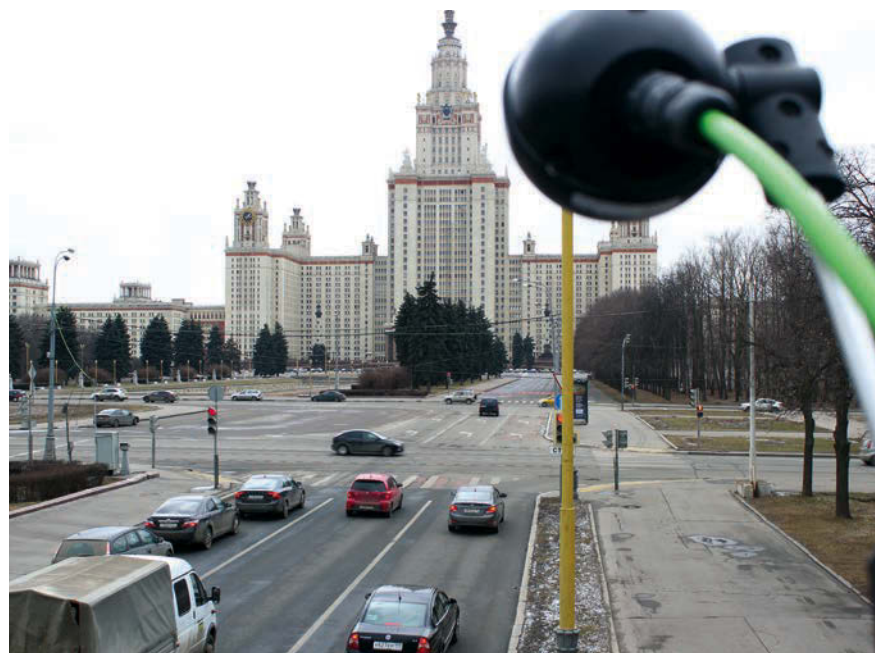
(Left) More than 3,000 TrafiCam x-stream sensors will be installed at traffic light controlled junctions (Right top) The device provides MPEG-4 or H.264 streaming color video at full frame rate (Right bottom) The sensor combines a CMOS camera and video detector
