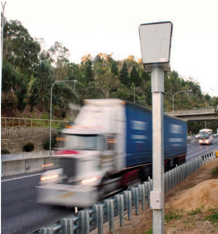
(Left) New fixed cameras in Australia can operate in a variable speed environment, distinguishing trucks from cars
