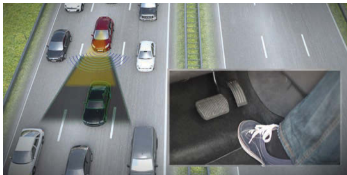
(Far left) The 2015 Ford Focus Electric is part of the company's move to alternative fuel types (Left) Ford's Traffic Jam Assist takes over braking and steering duties when its forward-looking radar detects traffic ahead
