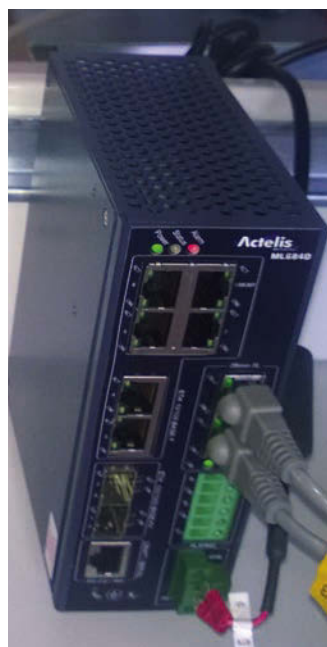
(Above) Effective infrastructure network design (Left) The ML684D is compact and fanless
