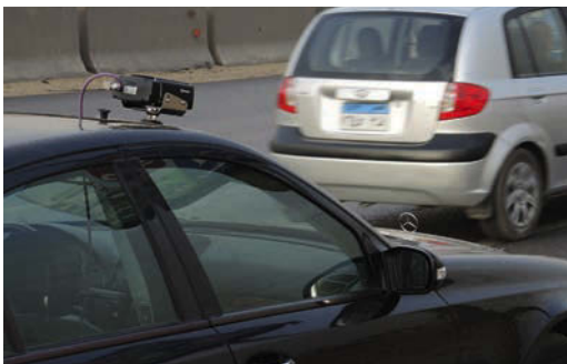
(Above) Tattile ANPR Mobile can be attached to the roof of a car (Left) It is an ideal tool for surveillance and security (Below) The device can capture clear images of fast-moving objects
