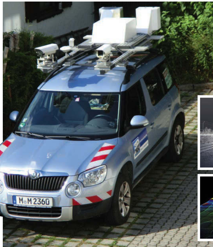
(Left) Figure 1: MoSES III mounted to a vehicle (Below) Figure 2: An example of a laser scanner point cloud (Bottom) Figure 3: A Belgian block test track transformed into a 0.005m curved regular grid
