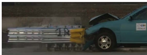
(Top) Tau crash cushions are redirective and bidirectional (Above and left) Excellent impact performance (Below) Aluminum alloy provides an environmentally friendly solution
