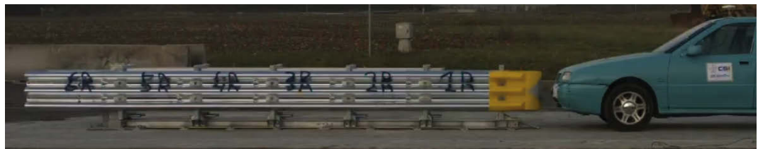
(Top) Tau crash cushions are redirective and bidirectional (Above and left) Excellent impact performance (Below) Aluminum alloy provides an environmentally friendly solution
