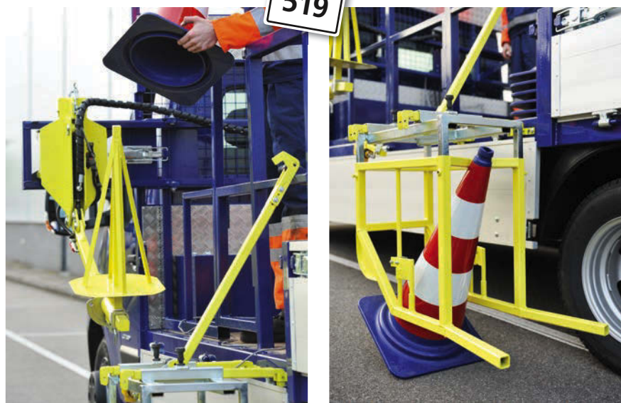
(Far left) Workers remain in a safe position throughout the cone placing task (Left) The Gerard machine places the cones at a preset distance
