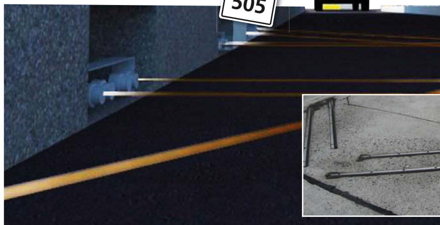
(Left) Light beams crossing the road (Below) Old-fashioned pressure detector for wheel size
