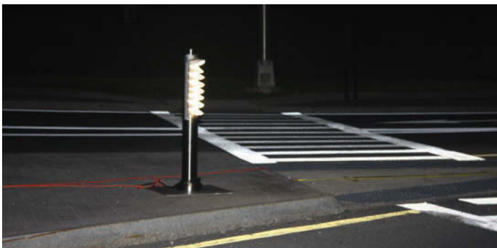
(Left and right) A novel bollard-based approach was adopted in tests by the Lighting Research Center as an economical and viable way to increase crosswalk safety and visibility
