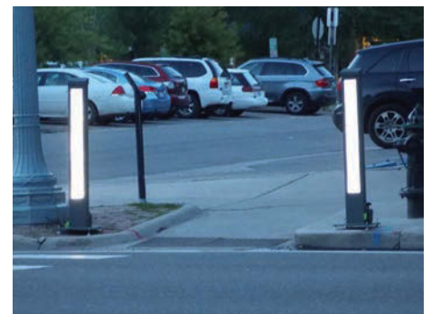
(Left and right) A novel bollard-based approach was adopted in tests by the Lighting Research Center as an economical and viable way to increase crosswalk safety and visibility
