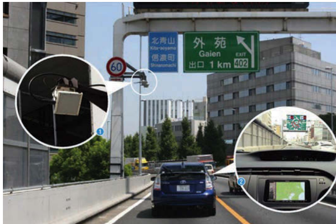
(Above) ITS Spots have been installed at more than 1,600 locations in Japan. The three basic services include dynamic route guidance, safety driving support and ETC (Right) Pioneer's Carrozzeria ITS Spot-compatible navigation device (Main) An increasing number of car makers are incorporating ITS Spot navigation systems as standard
