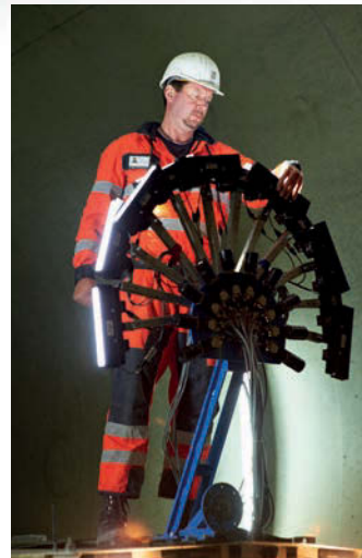
(Main) The pilot area scan camera (Above) The tCrack system at work in a Swiss tunnel (Left) An engineer sets up cameras and lighting
