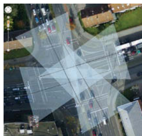
(From left to right) How the intersection is tracked with a detail camera, a radar and an overview camera
