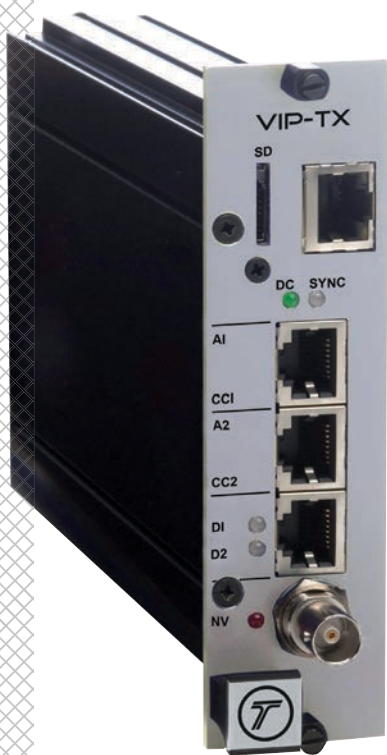
The VIP-TX (left) generates traffic data and incident detection information (Main) The technology supports operators with alerts on stopped vehicles, wrong-way drivers, pedestrians, lost cargo, smoke and traffic flow data
