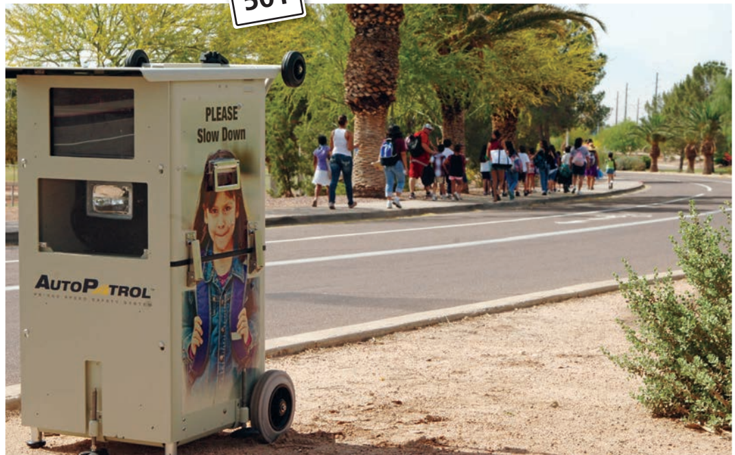
The Auto Patrol system uses 2D radar technology to identify vehicle speed
