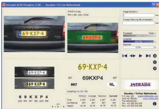
Effective OCR software allows license plate data to be captured
