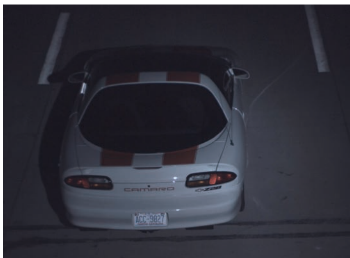
The goal of night lighting is to illuminate both vehicle license plate and scene without blinding or distracting the driver
