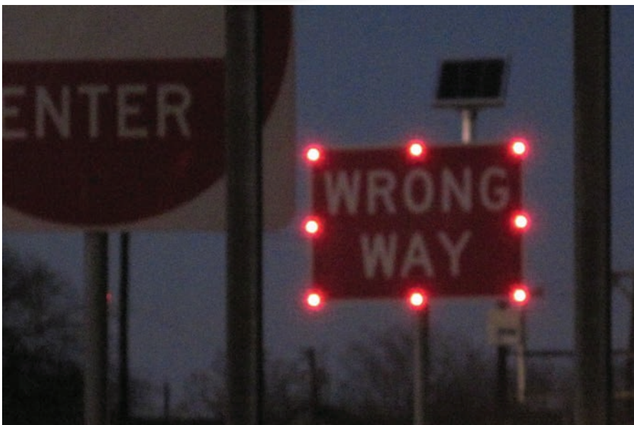
(Top right) According to the Texas Transportation Institute, lowering the mounting height of ‘Do Not Enter’ and ‘Wrong Way’ signs may be an effective countermeasure for preventing wrong-way entries onto highways (Below) A wrong-way vehicle triggers this system, turning on a ‘Wrong Way’ sign with flashing red LED lights
