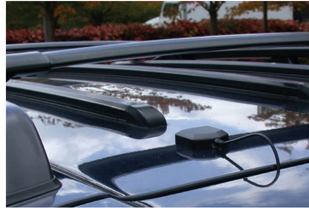
The GPS receiver, as used in the 2007 Oregon RUC trial
