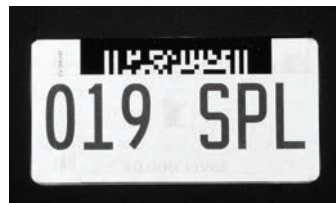
(Above) Barcode plate image taken in diffuse room light (Left) Image taken in infrared. Visually inconspicuous barcodes appear under infrared
