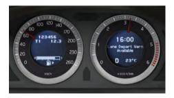
(Left) Volvo's LDW uses a camera system to recognize lane markings, sounding an alert if the driver strays out of the lane (Below) For drivers, Lane Assist can feel like hitting a rumble strip even though no such strip exists
