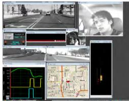
(Above) UMTRI analyzed all the data collected, including information on IVBSS system, driver and vehicle performance, as well as vehicle location and driving environment (Above left) Sensor coverage on the light vehicle fleet
