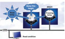
with gold electrodes and under consideration of the water film thickness and the temperature; and road surface condition (dry, ice, wet, slush) measured by the dielectric characteristics of the cover.
