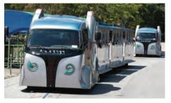
The OLEV is remotely charged via electromagnetic fields created by electric cables buried beneath the road
