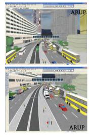
Legion for Aimsun was used to conduct pedestrian and vehicle modeling and Legion, enhancing the modeling functionality from a user perspective with robust improvements. These include boarding and alighting interaction between pedestrians and vehicles, vehicles giving way to pedestrians at cautionary crossings, and modeling results in 3D and enhancing output graphics for advanced simulation animation.
