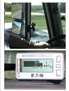
Lane-departure warning technology was combined with Eaton's radar-based technology in a fusion of data management and decision-making algorithms
