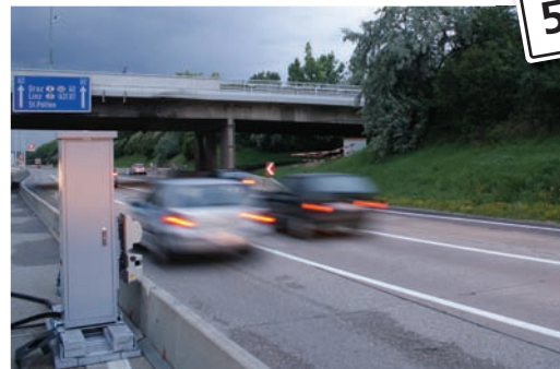
TraffiSection systems determine average speed on different stretches of road
