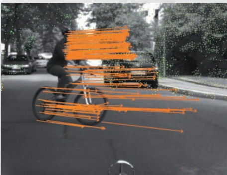
With Daimler's 6D vision technology, the pixels are not just measured spatially
