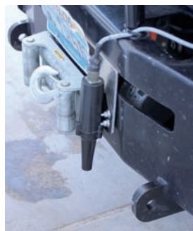
Trucks in the Nevada DOT maintenance fleet are to be fitted with mobile probes to fill in the blanks in the fixed RWIS network
