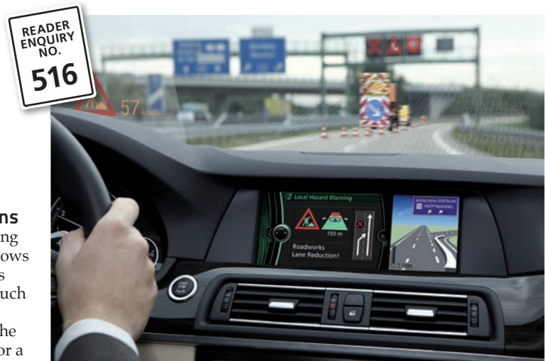
The driver receives LHW messages on the in-dash navigation device
