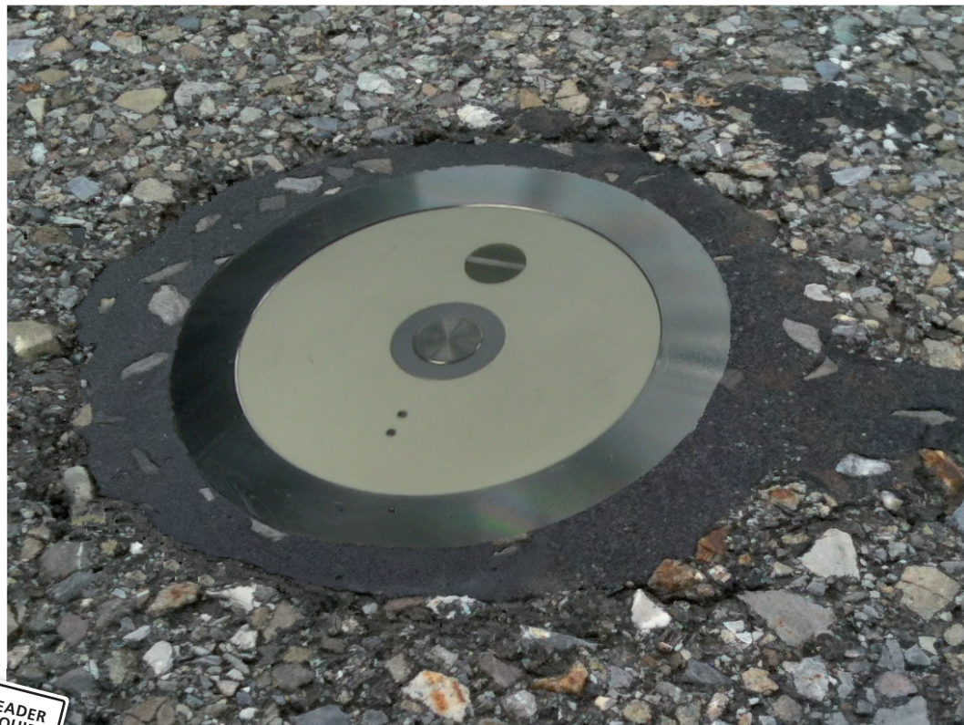
(Main) The new IT-Sens pavement sensor (Left) Screenshot from test data within the Borra-WEB MDSS system used by ASFINAG in Austria
