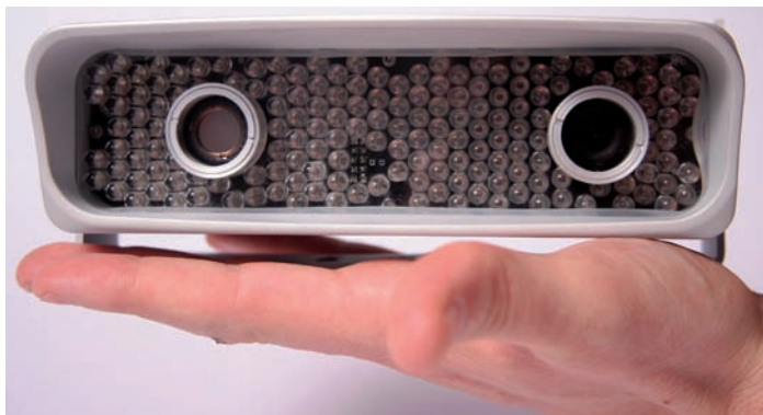
(Left) The complexity of reading Japanese plates (Below) Digital Recognition's iSharp ALPR camera
