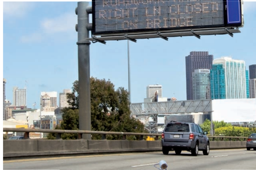
(Above) The PTC uses VMS to provide traveler information (Right) Cameras at intersections keep a close eye on traffic
