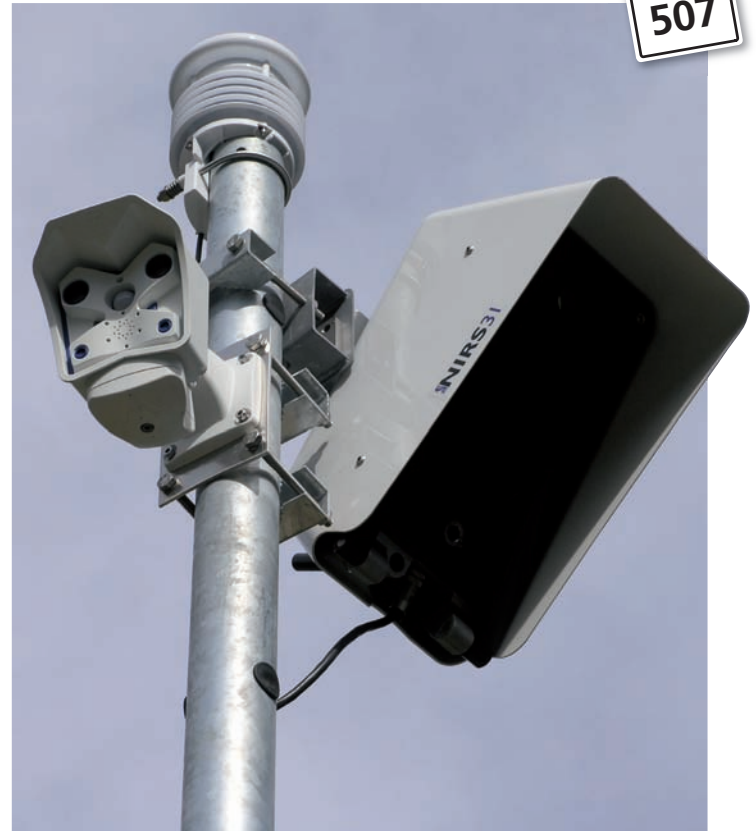
(Above) The NIR531 is a non-invasive pavement condition sensor (Right) It is easily installed at a number of locations where space is a constraint – including bridges and tunnels
