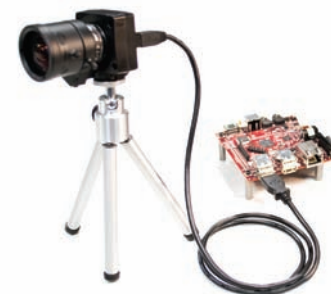
(Left and below right) The BeagleBoard is a USB-powered computer that easily connects to Chameleon cameras (Below left) Access control is one example of an ALPR application
