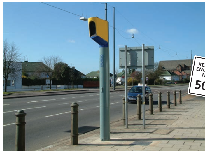
(Above) A stationary unit in situ (Left) One image captures all the evidence needed for verifying driving offenses
