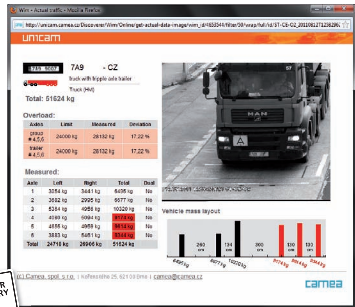
The UnicamWIM system captures all of the parameters needed for enforcement
