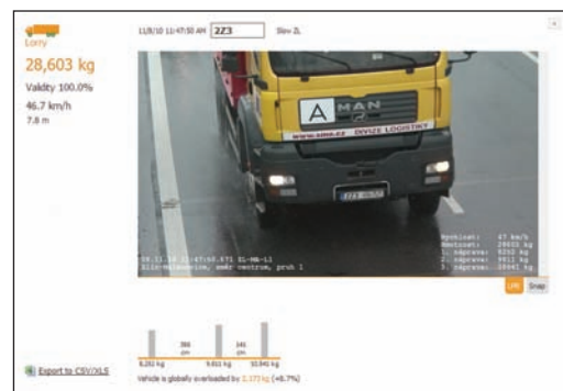
(Above) Raw data is processed and evaluated in a computer using advanced Cross algorithms (Left) Showing the vehicle detail via the CrossWIM system
