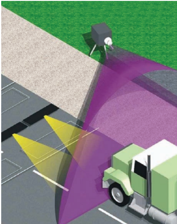
Another element that contributes to the increase of safety is the installation of a system measuring the depth of the tire profile
