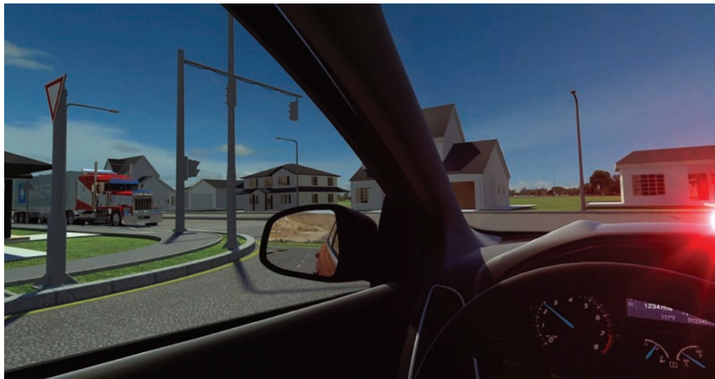
Once the in-vehicle computer receives data indicating a hazard, it can instantly warn drivers through visual and audio alerts
