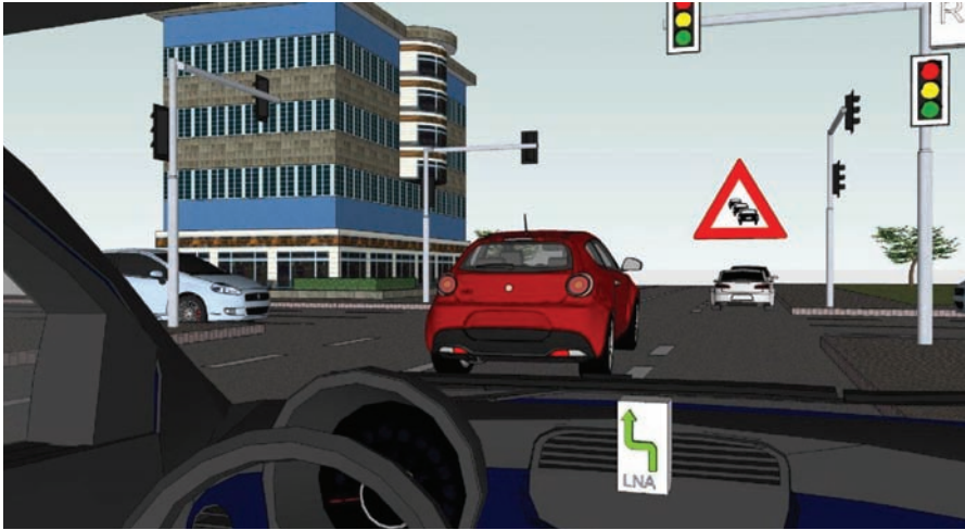
The Lane Navigation Assistant inside the vehicle will suggest to the driver a lane-change maneuver
