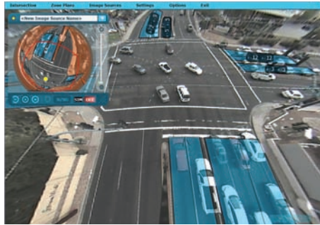
GridSmart from Aldis Inc couples an ultra-wide-angle camera for panoramic imaging of the entire intersection with advanced algorithms for real-time tracking of vehicle
