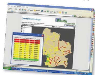
Chapman's route-based forecasting development involved the development of GIS models which utilized new survey techniques based upon GPS measurements and digital image processing
