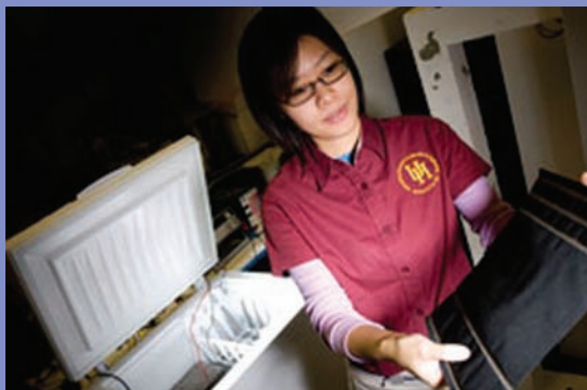
Christiana Chang holds a sheet of carbon nanofiber paper that she is embedding in concrete in an effort to create self-heating roads
