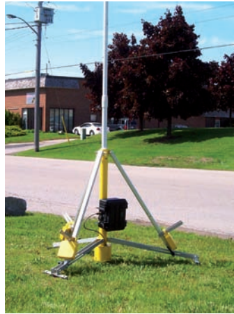
The tripod frame allows users to deploy the VCU at any location near the roadside
