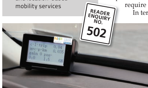
The OBU used in the Eindhoven trial featured a chipset from NXP based on ATOP
