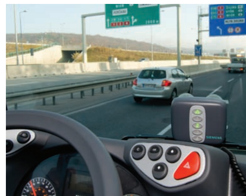
(Above) Toll data is continuously collected through the OBU using GNSS (Left) Around 65% of users are foreign trucks
