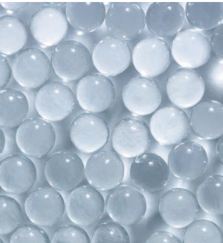
These titanium-stabilized beads extend the durability of reflective road markings far beyond the usual performance life
