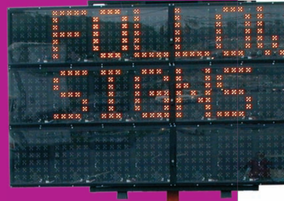
Portable dynamic message signs should be in operation prior to the PSE to alert citizens about the scheduled event
