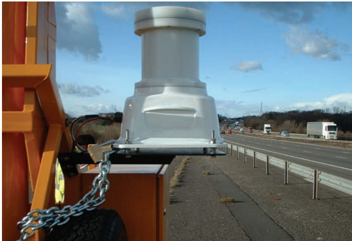
Navtech Radar's ClearWay uses high-frequency radar to scan the whole road surface, both up and down stream
