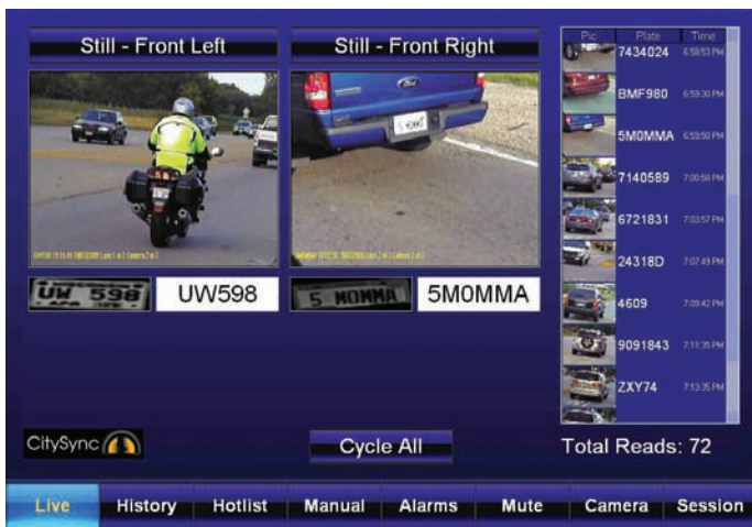
← A simple touch-screen interface gives full control of all vehicle cameras to a police driver with easy-to-interpret clear displays showing tracked vehicles and instant alarms with user-defined priority levels
