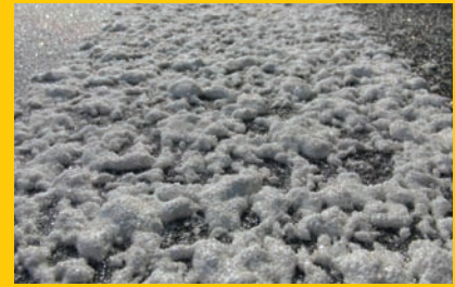
Cold plastics containing Degaroute reactive resin show less abrasion than other markings
