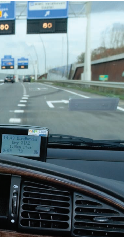
The OBU used in the Eindhoven trial, which features an NXP chipset
