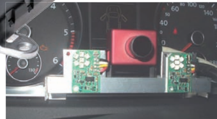
↑ Driver monitoring equipment will detect driver state (above) and a short-range 24GHz radar
