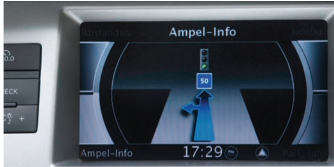
← Audi's Travolution project is exploring communication between vehicles and traffic signals
