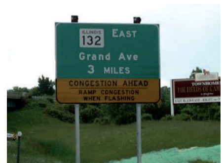
⤴ Illinois Tollway's I-94 queue warning system combines microwave detection at the start of the exit ramp with advance warning beacons
