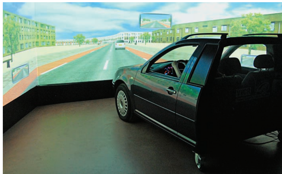
Figure 4: The fourth-generation VW Golf fixed-base driving simulator at TNO Soesterberg
