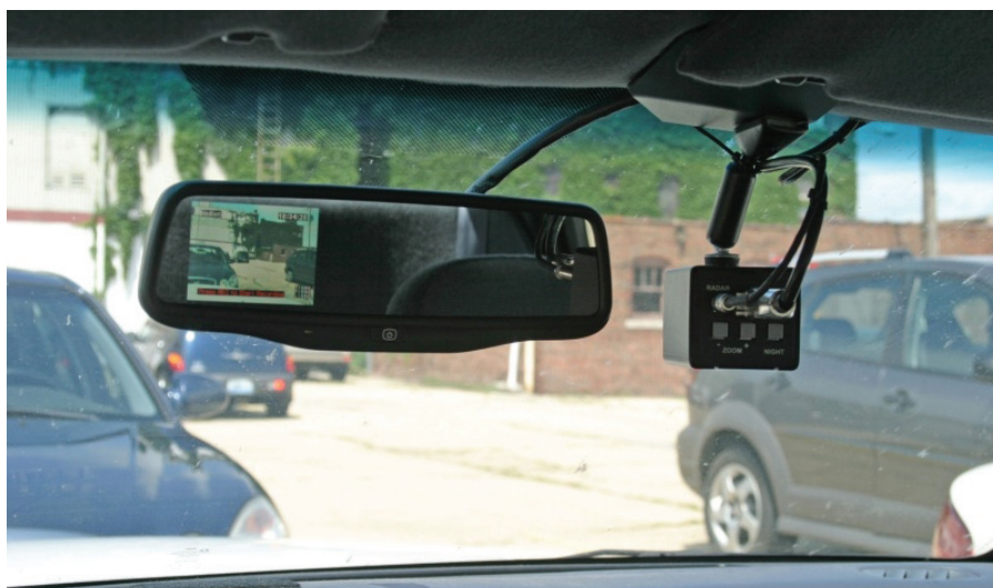
⦿ Decatur's LCD rearview mirror has a space-saving, user-friendly video display incorporated
