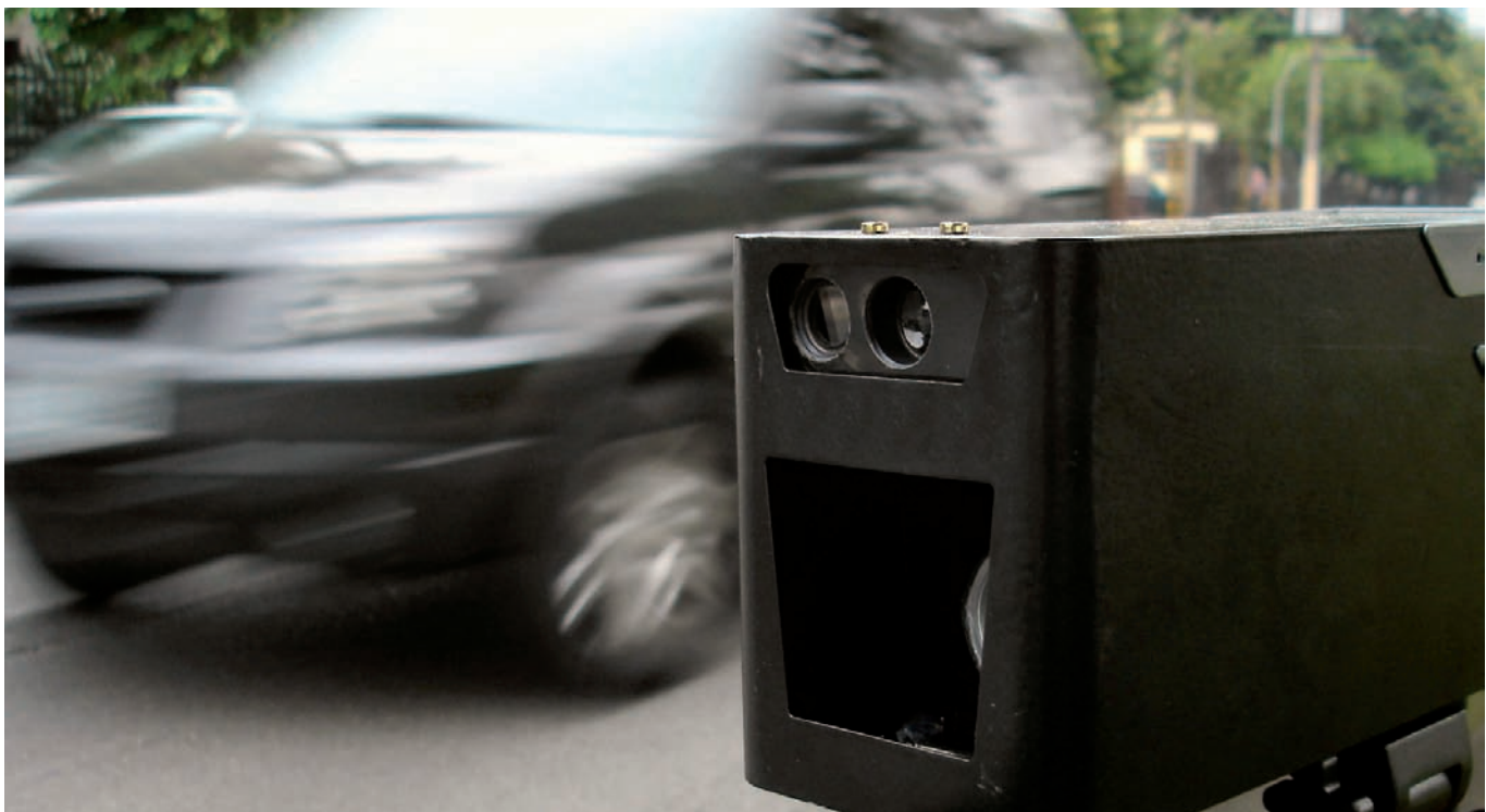
⦿ A portable speed measurement unit utilizing a more accurate and reliable laser technology can calculate the speed of vehicles over multiple lanes
