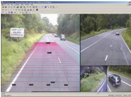
↑ To collect data for determining AusRAP Star Ratings, vehicles record photos of roads that form a 'video' of the network that can be streamed for analysis
