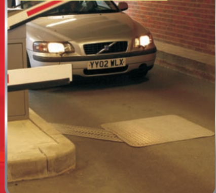
Vehicle Detection Pads Surface mounted directional vehicle detection loop pads
