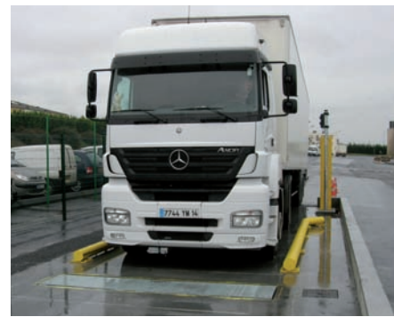
↑ The Captels system checks axle loads before vehicles are sent out onto the road, thereby reducing Carrefour's liability in case of accident
