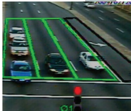
Autoscope video detection from ISS is ideal for signalized intersections, and is a cost-effective alternative to embedded loops
