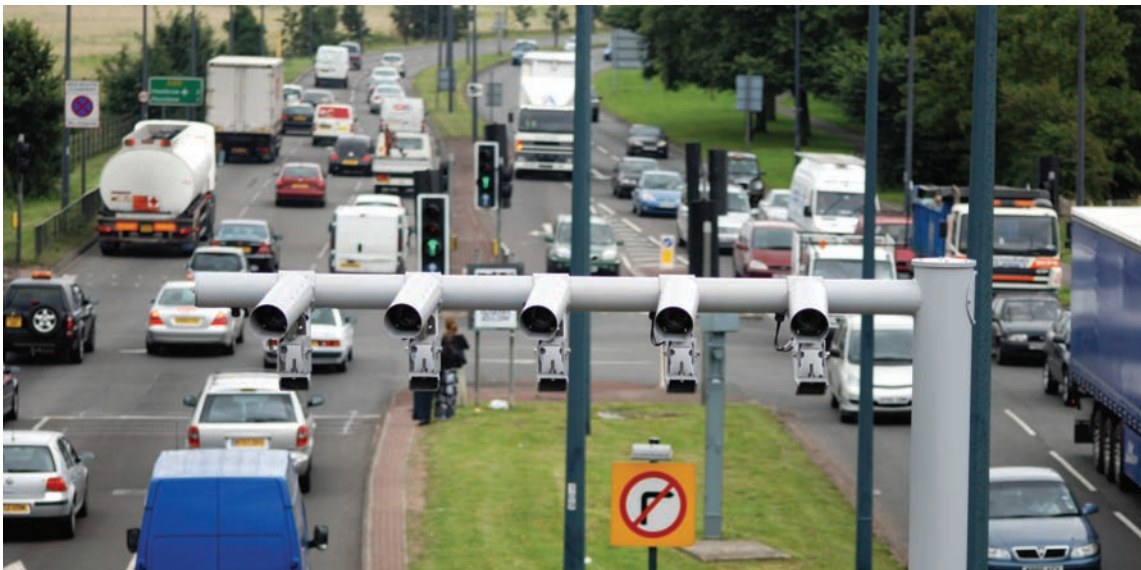
← Federal Signal's Spike cameras in situ in London, where they are used in the city's Congestion Charging Scheme
