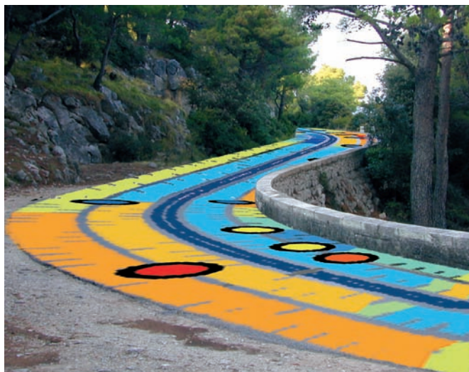
One of MARVin's results projected on the real road: skid resistance versus accident spots
