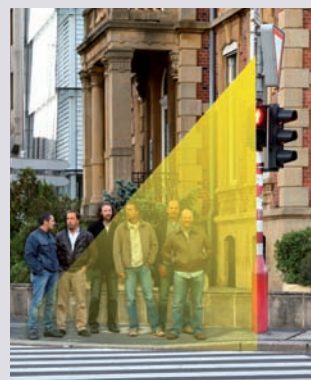
IEE's sensor works by emitting modulated infrared light that is reflected by nearby pedestrians
