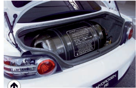
↑ A single hydrogen tank in the back of Mazda's 5/Premacy Hydrogen RE Hybrid
