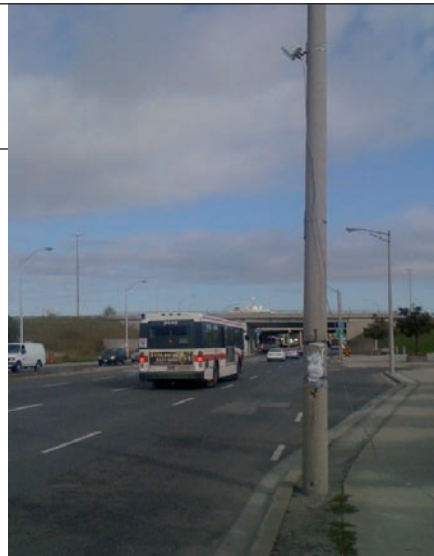
④ High concentration of vehicles in an urban scene ④ Figure 3: The RTMS detection system can be mounted on existing poles close to the curbside ④ Figure 4: Zero setback capability makes the RTMS an ideal solution for urban traffic control
